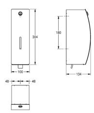
Soap dispenser for wall mounting, stainless steel, surface satin finished, front with InoxPlus surface refinement for the reduction of finger marks and better cleaning characteristics (easy to clean), material thickness 1.5 mm, curved front cover, cylinder lock with Franke standard key, inspection window on front, suitable for liquid soaps and lotions, 0.8 liter soap tank, with plastic pull lever, includes stainless steel screws and dowels.
