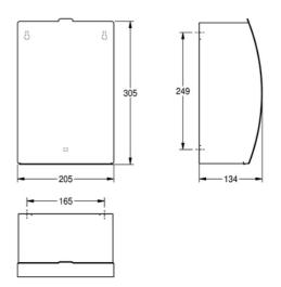
Sanitary towel and disposal bin for wall mounting, stainless steel, surface satin finished, front with InoxPlus surface refinement for the reduction of finger marks and better cleaning characteristics (easy to clean), material thickness 1.5 mm, curved front cover, approx. 3.8 liter capacity, folding selfclosing lid with piano hinge, removable plastic container inside, incl. stainless steel screws and dowels.
