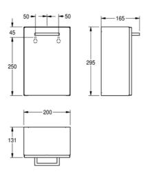
Sanitary towel and disposal bin for wall mounting, stainless steel, surface satin finished, material thickness 0.8 mm, folded front cover, approx. 3.7 liter capacity, removable plastic container inside, incl. stainless steel screws and dowels.
